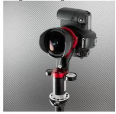
The imagery taken with Canon DSLR camera and fish-eye lens shooting in 4 directions.
